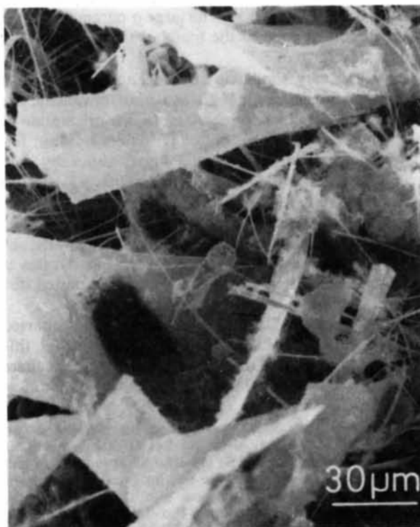
Fig. 5. Scanning electron microscope image of synthetic 'cannizzarite'. The larger, bladelike crystals are cannizzarite, whilst the finer material is a mixture of cannizzarite and bismuthinite, \text{Bi}_2\text{S}_3 . The extreme thinness and fragility of the crystals is evident in this image; most crystals are bent and the cannizzarite is both frayed and transparent to the 20 kV electrons used in this study.
